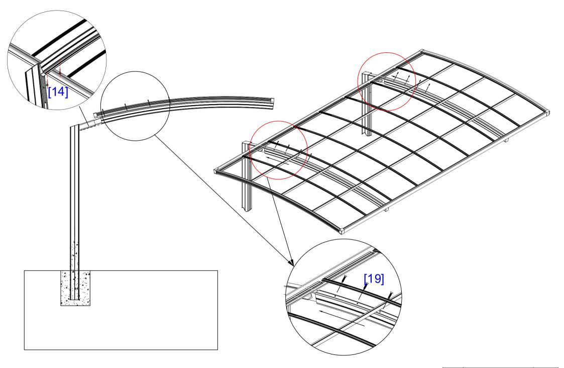
STEP9: Install bigger support tube caps, front tube caps.
