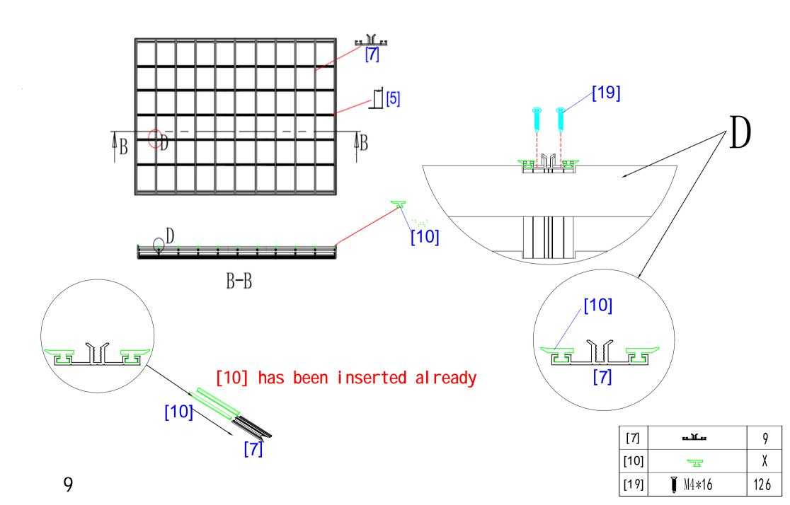
STEP5: Install pc sheet channels.
