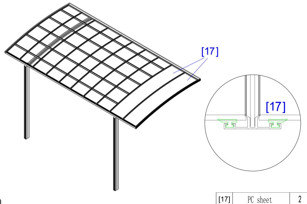
STEP11: Install top cover strips. Screw 25 and screw 26 are used interchangeably.
